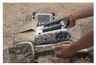
(MTGR)" out of your backpack and sends it up the stairwell. Weighing 13lbs. the MTGR is the lightest UGV around with the capability of climbing stairs. MTGR has been developed for intelligence gathering and counter-IED (C-IED) operations. It stands out due to its light weight, high maneuverability (can climb stairs), and its abilities to overcome 60 degree obstacles.
