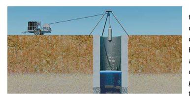
The AIG is used all over the world to rehabilitate water wells with dropped capacity. The design consists of the patented impulse generator, high pressure hose reel, control panel and one or more compressed nitrogen or air cylinders. As the compressed gas feeds through the hose and into the Impulse generator, pressure builds
