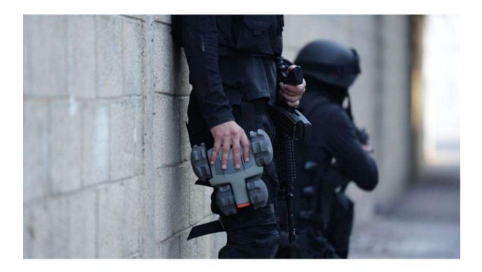
Weighing less than 2 lbs. and made from an extremely strong composite material the IRIS was been designed to be thrown behind walls and withstand large drops thereby making it easy for you to deploy. The robot even includes a sling on its side (a wire that allows the IRIS to be flung
