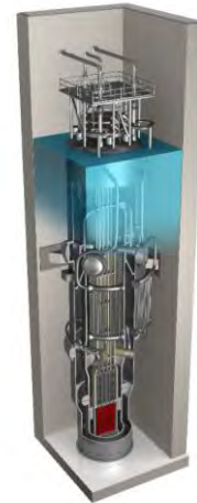
Figure 24. NuScale Power Module (courtesy of NuScale)
